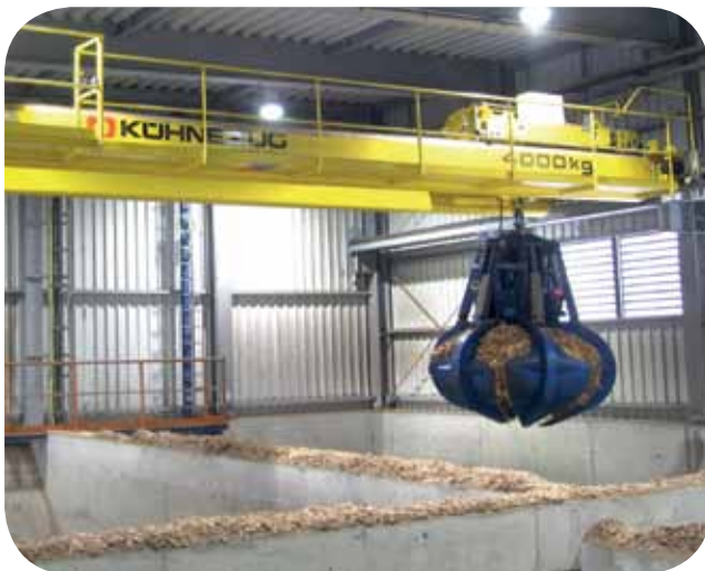
4 t / automated with grab / high speeds
