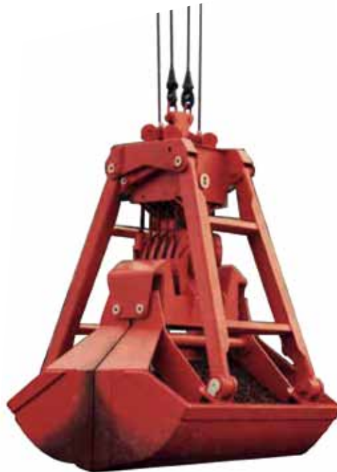
10 t clamshell rope grab for coal handling
