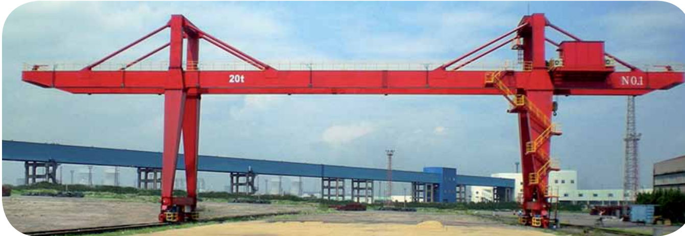
20 t / 40 m Span / RMG + boom
