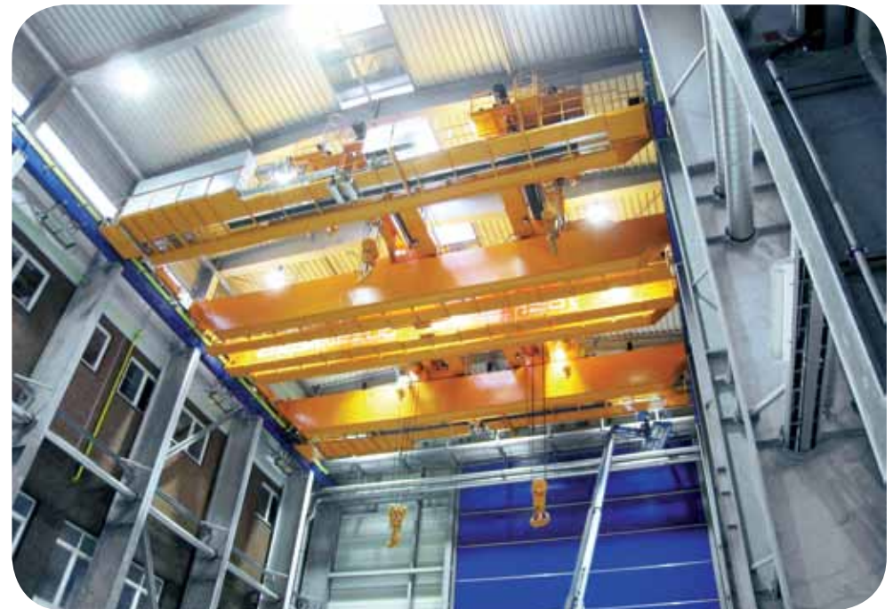
2 x 120 t = 240 t / full tandem / submarine production
