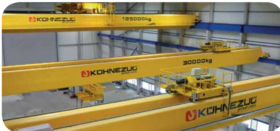
2 x 125 t = 250 t tandem function of two cranes / 30 t / 30 t / span 35 m / HOL 15 m / offshore wind turbines
