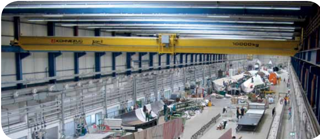
10 t / span 23,8 m / HOL 11 m / rotor blades for wind turbines
