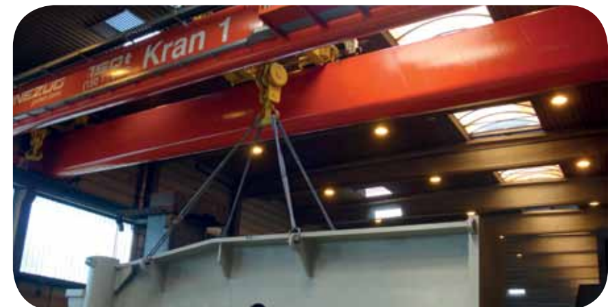
150 t / span 31 m / HOL 10 m / machine construction
