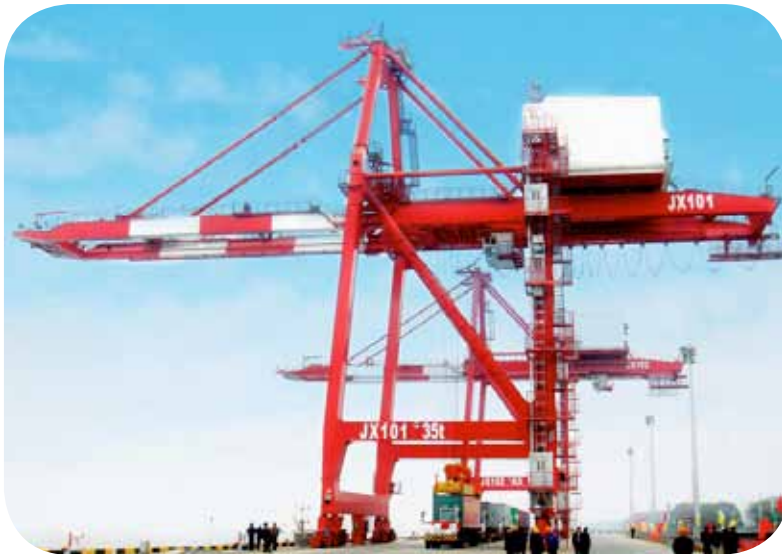
STS Container Cranes with capacities up to 65 t
