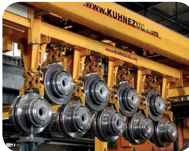
40 t / automated steel mill crane
