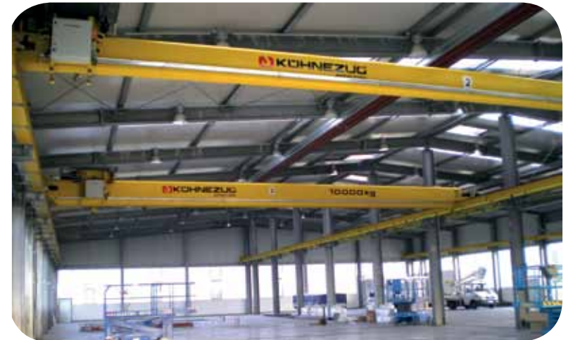
10 t / span 22,7 m / HOL 11 m / machine construction
