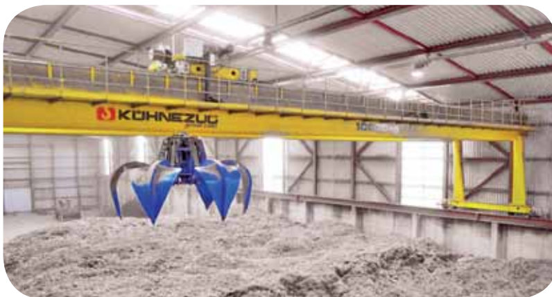
10 t / span 35,25 m / automated with grab
