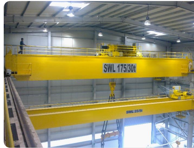
KÜHNEZUG – Double Girder Crane with 175/30 t Capacity.
