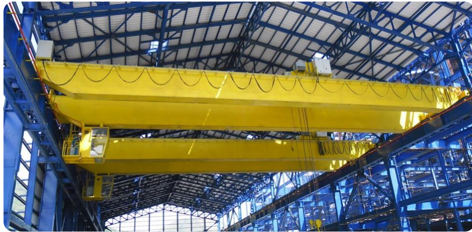
KÜHNEZUG – Double Girder Crane with 100 t Capacity.
