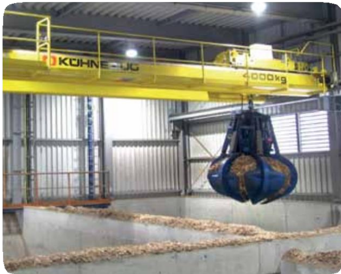
4 t / automated with grab / high speeds
