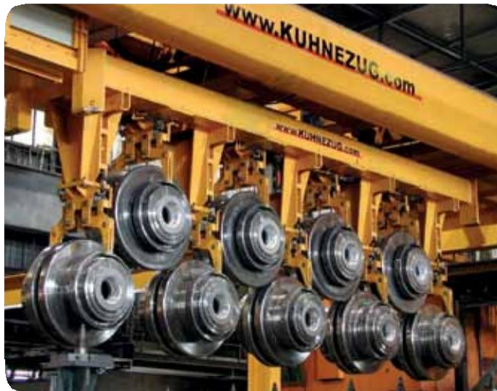
40 t / automated steel mill crane
