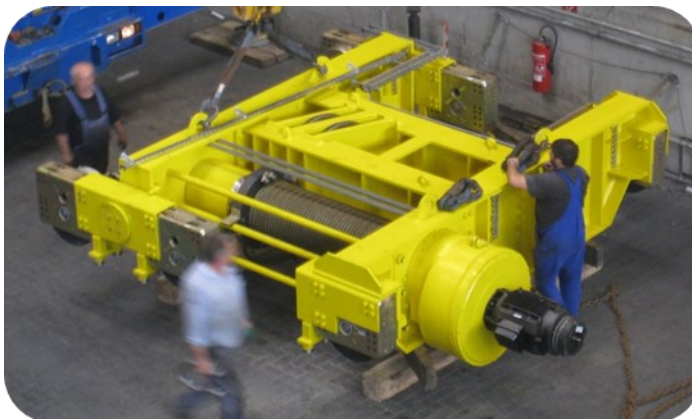
150 t load capacity with a trolley height of only 900 mm
